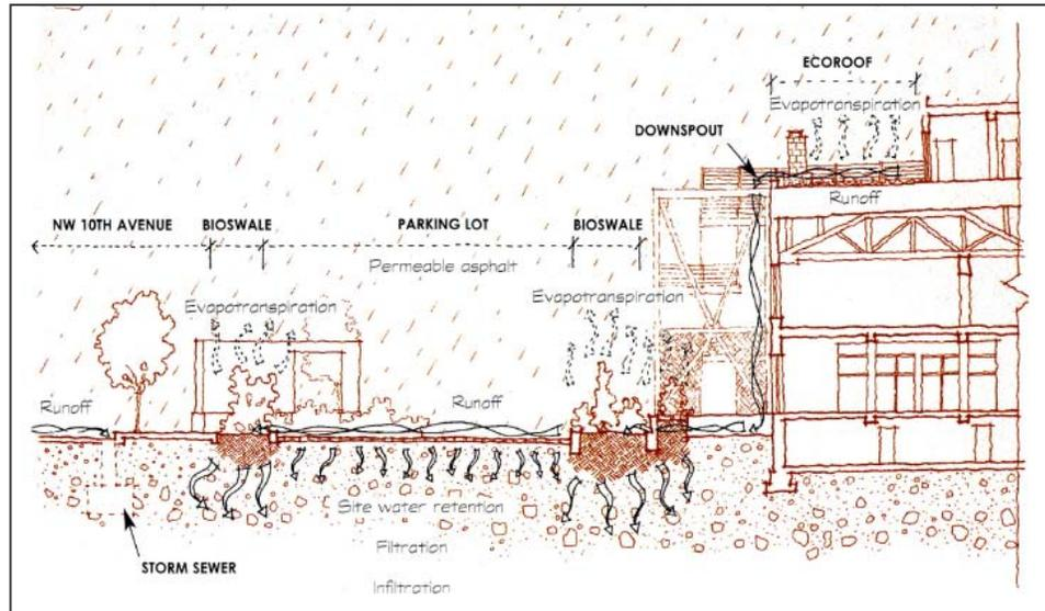
Figure 8c: Illustration of rainwater infiltration in the Natural Capital Centre parking lot
