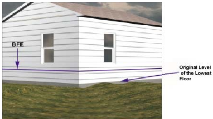
Technique 2 Convert the existing lower area of the house to nonhabitable space and build a new second story for living space.
