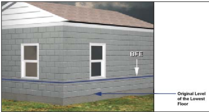
Technique 1 Extend the walls of the house upward and raise the lowest floor.
