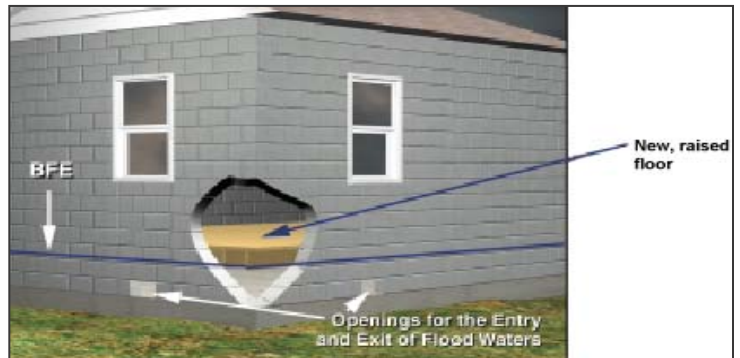
Technique 1 Extend the walls of the house upward and raise the lowest floor.
