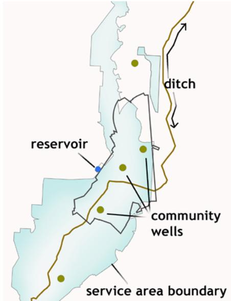
Figure 1: Community wells and a balancing reservoir provide water to most of the town.
